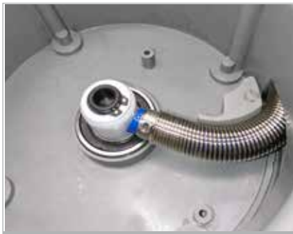
Kink protection with fixation to protect against jerky hose pull-out
