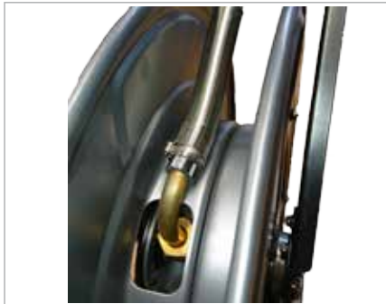
Quick detachable and refittable main hose for easy maintainability
