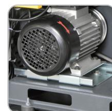
*Belt tensioner skid that adjusts the tension of the belt and facilitates its replacement.*
